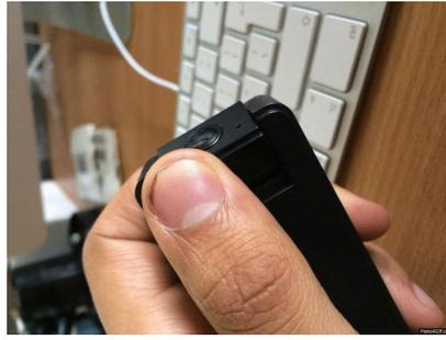
The Adjustable head can be tilted 180 degrees. This can be done by lightly applying pressure on the camera until it moves.
